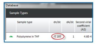
The refractive index for a series of 5 concentrations of polystyrene provided by Malvern was measured with a Rudolph J457 Laboratory Refractometer. The results are shown below. The results are nearly perfect, with a correlation coefficient of 0.999 and a measured value of 0.188, or 1.6% higher than the provisioned value.
